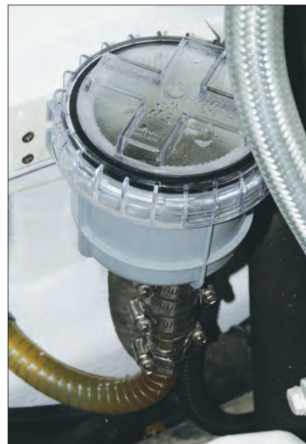
Far left —Even though most internal strainers are not this murky, you usually have to remove the lid to see what's in the basket. Left —A more modern version affords a better view to easily assess fouling—without actually opening the strainer.
